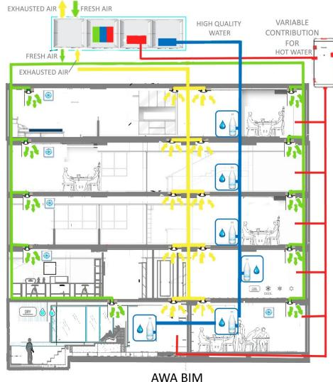
Integrated system for WATER from AIR production and active Thermal Energy RECOVERY for ventilation systems
